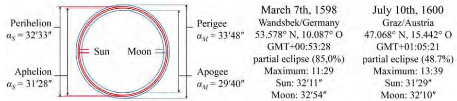
FIG. 3. Left: Periodic variations in the solar and lunar angles due to the eccentricity of the Earth's and Moon's orbits. *Perihelion* (January) and *Aphelion* (July) are the closest and furthest points of the Earth's orbit around the Sun. *Perigee* and *Apogee* are the closest and furthest points of the Moon's orbit around the Earth. Right: Reconstructed data on the solar eclipses observed by Brahe 1598 and Kepler 1600.<sup>20</sup>
