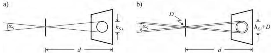
FIG. 2. a) Relationship between image size  $h_{S,i}$ , image distance  $d$  and solar angle  $\alpha_S$  for ideal pinhole imaging, i.e. expansion-free aperture. b) If the influence of aperture  $D$  is taken into account, the solar image is enlarged.
