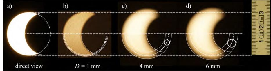
FIG. 12. Influence of the pinhole on the size of the solar image for different pinhole sizes  $D$  (b-d) compared to the scaled direct view of the partially eclipsed 'Sun' (a). Images b-d have been mirrored to facilitate comparison. The measurement uncertainty of  $h_S$  and  $h_M$  is in the order of  $\pm 1$  mm.
