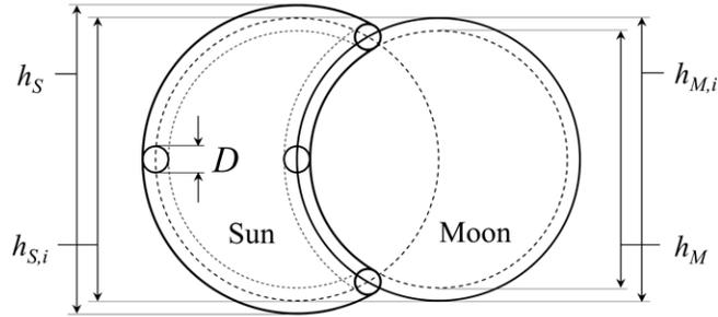
FIG. 6. Kepler's solution to the Moon puzzle: By convolving the image of the partially occulted Sun with the imaging aperture  $D$ , the solar image  $h_S$  appears enlarged ( $h_S = h_{S,i} + D$ ) and the lunar image  $h_M$  reconstructed from the concave edge appears reduced by the same amount ( $h_M = h_{M,i} - D$ ). For simplicity, the size of the images of Sun and Moon are assumed to be the same.
